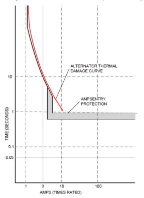
Short circuit shutdown (51) - Output current on any phase is more than 175% of rating at time of shutdown. The control replicates the function of a 51V relay by discriminating between short circuit conditions and shutdown conditions, and shutting down the genset as fast as is necessary on a short circuit condition while operating as long as is possible on an overload condition. Control includes algorithms to protect alternator from repeated over current conditions over a short time.
