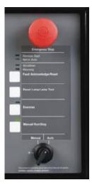
**Off/manual/auto mode control switch** - The *not* in *auto* lamp will flash when the control is in the *manual* or *off* mode. In the *auto* mode, the generator set can be started using the exercise push-button or with a start signal from a remote device, such as automatic transfer switches.
