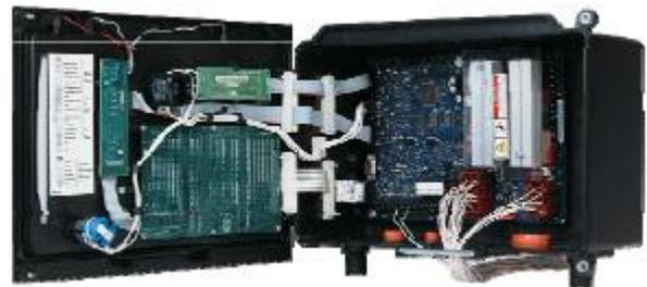
**High coolant temperature shutdown** - Level is preset to match the capabilities of each engine. Control includes time delays to prevent nuisance shutdown signals.
