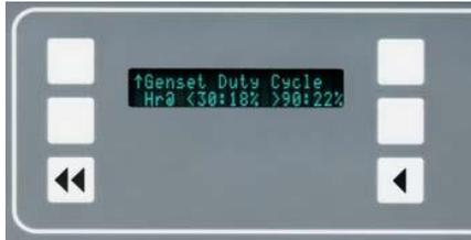
**Load profile data** - Control logs data indicating the operating hours at percent of rated kW load in 10% increments. The data is presented on the operator panel based on total operating hours on the generator set based on number of hours under 30% load and number of hours at more than 90% of rated. InPower can be used to read data in detail (10% increments).
