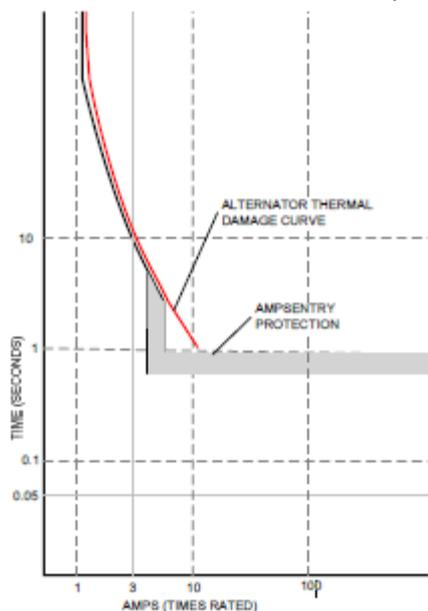
**Short circuit shutdown** - Output current on any phase is more than 110%, more than 175% of rating, and approaching thermal damage point of alternator. Control includes algorithms to protect alternator from repeated over current conditions over a short period of time.
